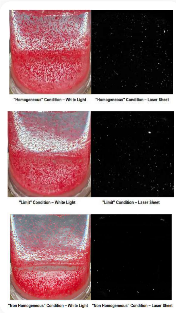
FIGURE 3 Illustration of the three visual conditions determined in the 45 mm vessel: Homogeneous, Limit, and Non-homogeneous. The left panel presents visual results and the right panel presents laser imaging results. The tests were conducted using model beads of 355–425 \mu\text{m} (mean size \sim 400\mu\text{m} ), with a tilt angle of 25^\circ and an H/D ratio of 0.7.
